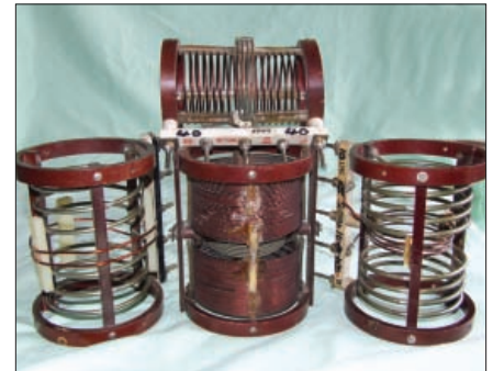
The coils are all of a common 100mm diameter, but with differing numbers of turns.
