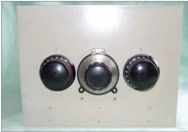
Three controls on the front panel, the two output capacitors flanking the input matching and tuning capacitor in the centre.
